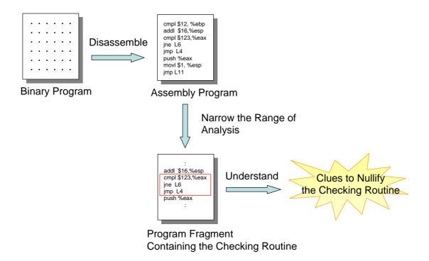
Figure 1.2. A scenario of obtaining clues to nullify the password-checking routine
